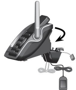
4. Plug the telephone line cord (or DSL filter) into the wall jack. Plug the power adapter into a power outlet not controlled by a wall switch. Align the slots on the back of the telephone base with the studs of the wall mounting plate. Make sure the telephone line cord does not get caught between the wall mount plate and the telephone base.
