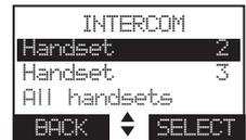
The call is automatically put on hold. The telephone base displays **Calling HANDSET X** or **Calling all handsets**. The destination handset(s) rings and displays **BASE 0 is calling**.
