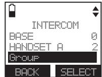
The call is automatically put on hold. Your handset displays **Calling HANDSET X**, **Calling BASE 0** or **Calling all devices**. The destination device rings and displays **HANDSET X is calling**, or **HANDSET X is calling all**.
